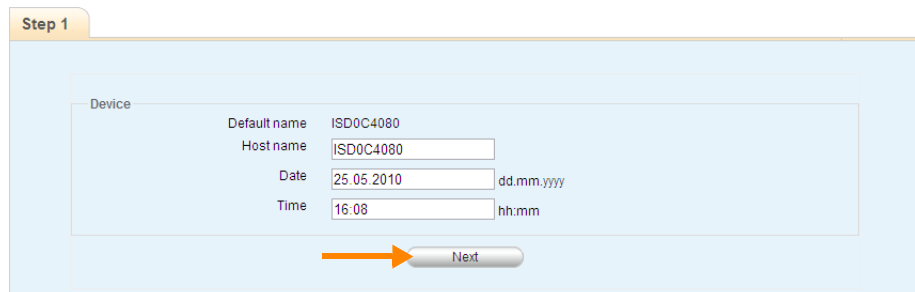
Illus. 5 Check host name, date, and time and click NEXT to confirm
