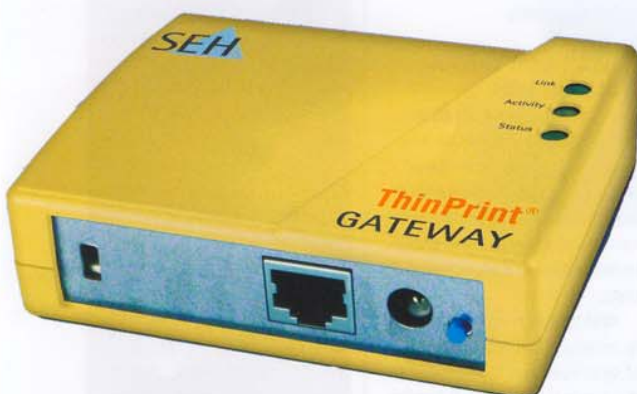
A typical gateway which can be used to protect data in a thin client network.
